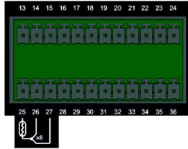
SENSORS. 8 inputs for RTD sensors, Pt100 type with three wires (max section 1.5mm<sup>2</sup>).
