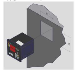
Fix the unit securely with the blocks supplied.
