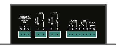
1048 BASIC The control unit has UNIVERSAL POWER SUPPLY, it can be supplied by 85 to 260 50/60Hz Vca-Vcc, irrespectively of polarity in Vdc (terminals 40-42). The ground must always be connected to terminal 41.
