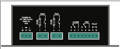
The 1048 ETH control unit has **UNIVERSAL POWER SUPPLY**, it can be supplied by **85** to 260 Vca-Vcc, **50/60Hz** irrespectively of polarity in Vdc (terminals 40-42). The ground must always be connected to terminal 41.
