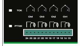
TCK SENSORS. Each temperature sensor TCK has a yellow conductor (+) and one red (-), connect the sensors following the image, example CH1 = 15 Red - 13 Yellow.
